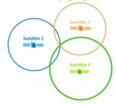
where all three circles intersect. Each satellite is at the center of a sphere with the GPS receiver found in the location where the satellites intersect.<sup>46</sup>
